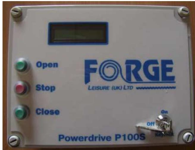
4. Using either the remote transmitter or pushbuttons, press the cover out button to deploy the cover then stop it by pressing the cover out button again when at hand height.
